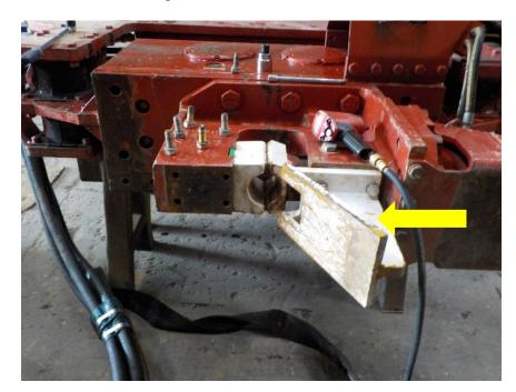
Using an auxiliary hydraulic power pack open the jaws and remove the fixed jaw (4050284)
