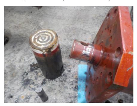
Install clamp slide pin (4200138) The pin will be marked with a T on one of the pin. This is the top of the pins taper. Strike or press the pin from the T end to install. Continue until flush
