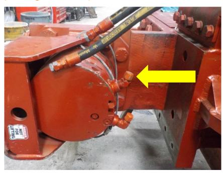
Remove the caps and plugs and reconnect the lines accordingly
