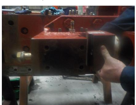
Install Fixed jaw bolts 1"-8 x7" (9016137)-2 places with lock washers (9030612) torque 600 ft.lbs
