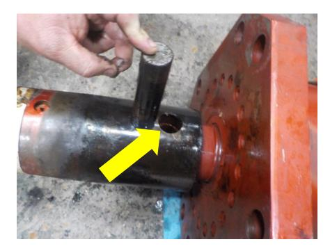
Install clamp cylinder with round clamp slide
