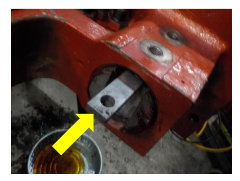
Remove 1  $\frac{1}{4}$ "-12 x 3" bolt (9016218)-6 places from clamp cylinder flange.
