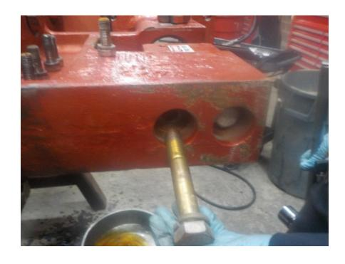
Install 3/4"-10 x 2" bolts (9015917)-4 places and lock washers (9030610) with short jaw guide (4051254) torque 250 ft.lbs
