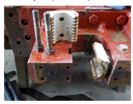
close the clamp and remove the roll pin (9240055) and standard V-5Esc moveable jaw (4050076)
