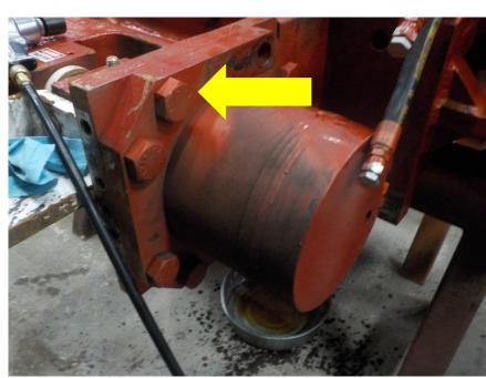
Remove the clamp cylinder with standard clamp slide from the clamp housing
