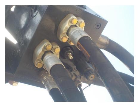
Check if any of the adjustable cartridges have been hit or damaged. This can change the pressure setting.
