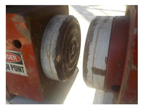
Inspect the chrome shaft on the side clamp cylinders for damage to the chrome
