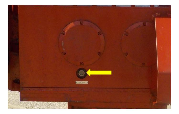
Check the hour meter located on the Junction box
