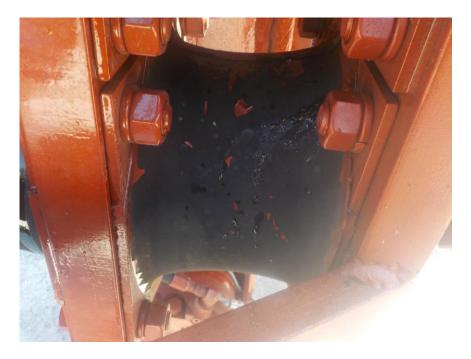
Also inspect the ones on the side clamp for damage such as nicks or tears
