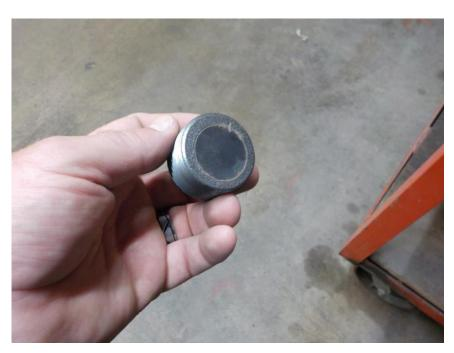
Apply a thread sealant to the pipe threads on the drain plug. This can be liquid Teflon or Teflon tape.
