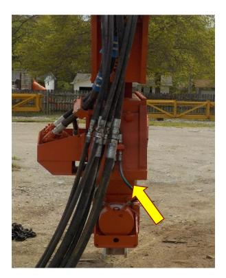
Fill exciter case with Shell Morlina S4 220 or equivalent. Approximately 5 gallons of oil.
