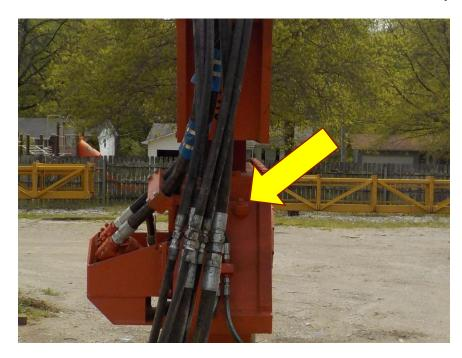
Next using the 15/16 inch 8 point socket remove both of the square drain plugs in the bottom of the Exciter case.
