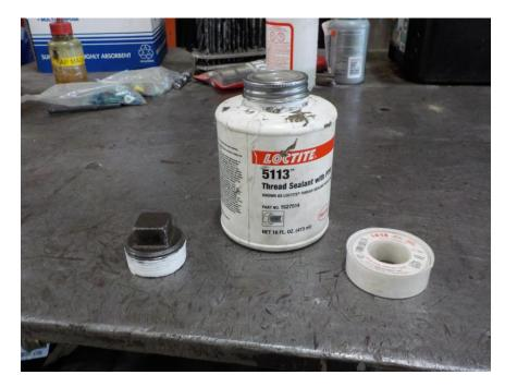
Place both drain plugs with sealant back into the bottom of the exciter case.
