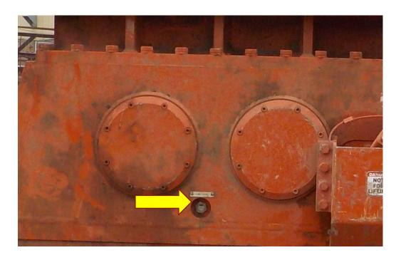
Replace the fill plug with the preferred sealant on the pipe threads.
