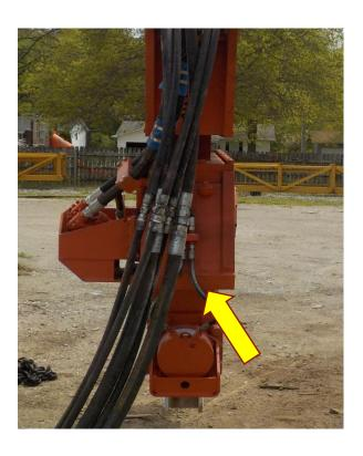
Clean the drain plug and wipe off the magnet that is on the inside.
