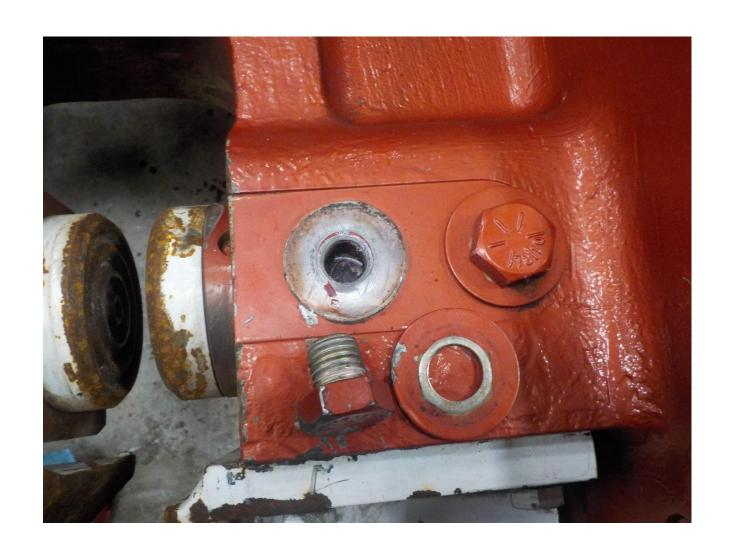
Remove clamp cylinder from the clamp housing
