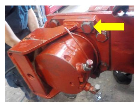
Install the bottom bolts (9015917) apply Loctite and torque to 250 ft. lbs.
