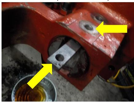
Once you have the slide key installed correctly you can install the slide key bolts (4050091)-2 places without flat washers
