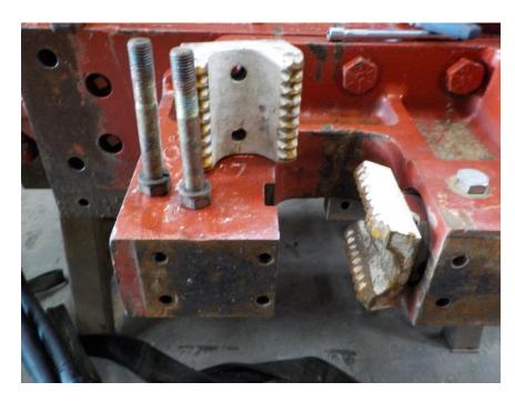
Install tall jaw guide (4050134) using the same bolts (9015917) and lock washer (9030610) from the other jaw guide. Torque to 250 ft. lbs.
