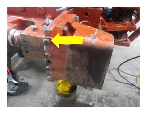
Install slide key (4050089) into appropriate slot on jaw guide making sure to line hole up for slide key bolts
