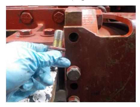
Remove 1  $\frac{1}{4}$ "-12 x 3" bolt (9016218)-6 places from clamp cylinder flange.
