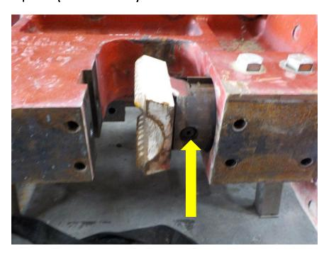
Open the clamp and install the fixed jaw (4050284) using the proper hardware (9016137) bolt and (9030612) lock washer. Apply Anti-seize to the jaw bolts and torque to 600 ft.lbs
