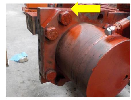
Install clamp cylinder guard using (9016224) long bolts apply anti-seize and torque to 1,500 ft. lbs.
