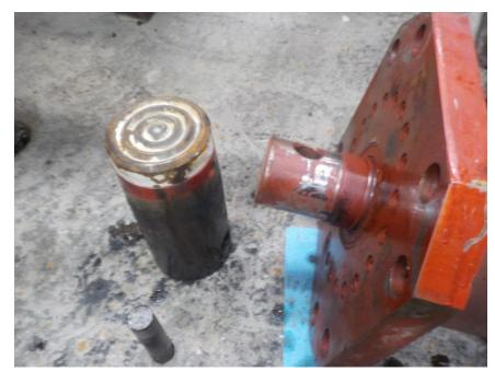
Install standard clamp slide (4050311) over the cylinder rod and line up the holes
