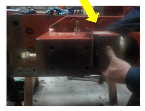
Install clamp cylinder with standard clamp slide
