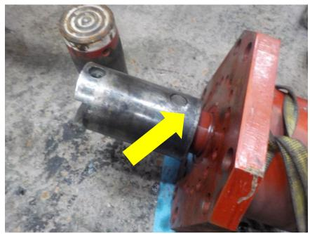
Remove ¾"-10 x 2" bolts (9015917)-4 places to remove moveable side jaw guide (4050134)
