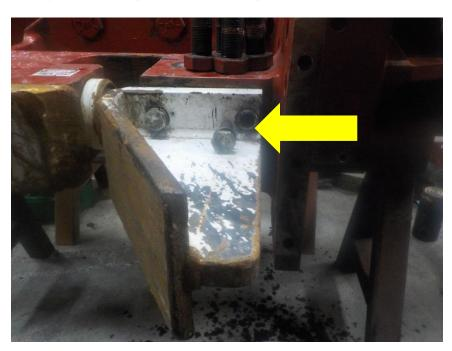
Remove 3/4"-10 x 2" bolts (9015917)-4 places to remove fixed side jaw guide (4051254)
